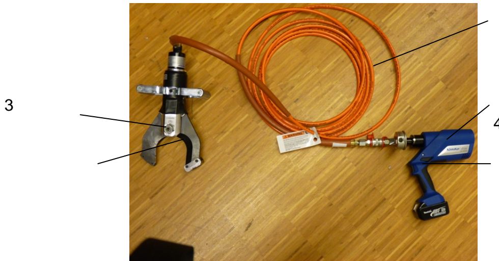
Fig. 1: Example of a motor-operated cable cutter
